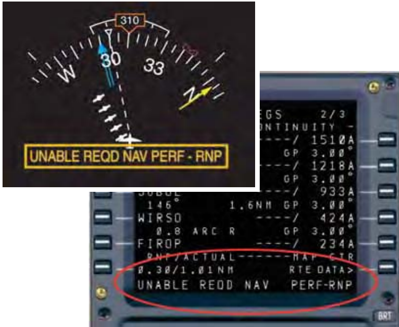
Figure B-3. An alerting system in the pilot's primary view must warn if ANP exceeds RNP. This alerting system is comparable to an "OFF" flag for a VOR or ILS.
